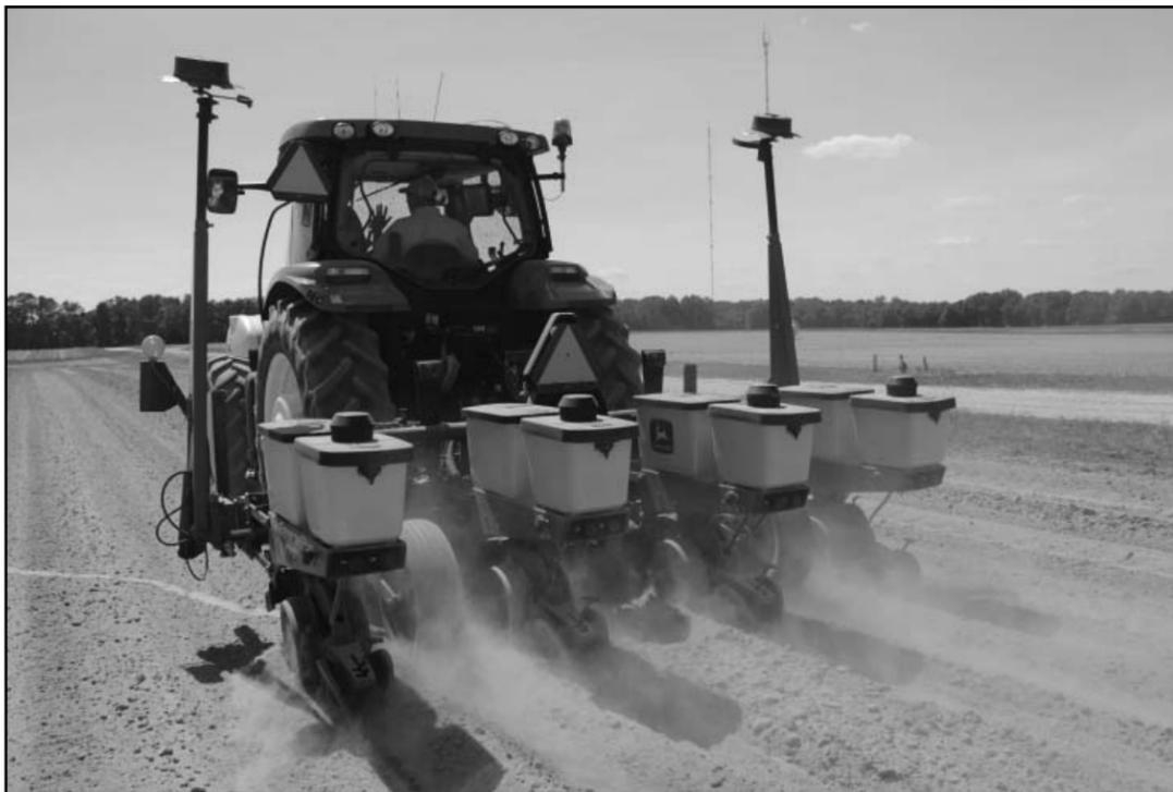
At left, a worker at Central Crops Research Station in Clayton demonstrates planting with an auto-steer tractor. Inside the cab of the tractor, you can see his hand is off the steering wheel.
