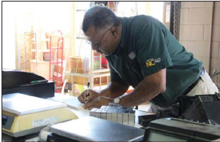
Standards Division inspector Ben Foster checks scales at the State Farmers Market in Raleigh. He determines the accuracy of the scales by placing known weights on the scale and recording the weight the scale notes. If there is a discrepancy of more than .03 pounds, the scale must be calibrated.
