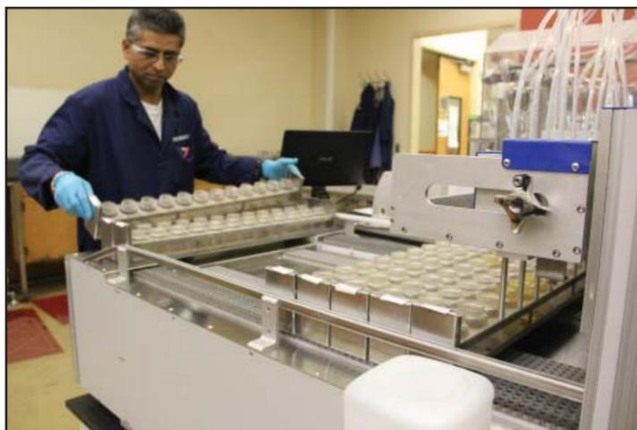
**Rohan Mohammed, a chemistry technician, loads the custom-designed automated dispensing unit that adds solutions to extract soil humic matter and plant available nutrients.**
