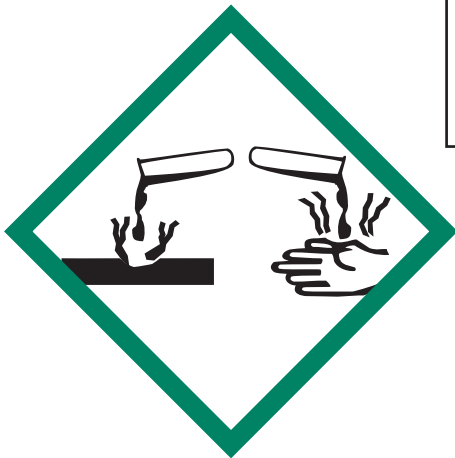
CORROSION: SKIN, EYE OR METAL
