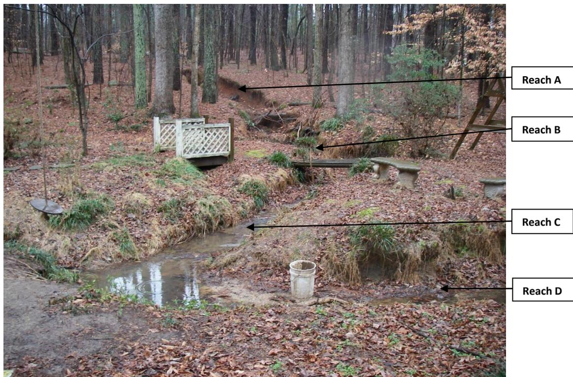
**Reach A:** 75 ft long by 3.5 ft high by 0.75 ft deep (9 inches), both banks eroding, average bulk density, eroded over a 6 month (0.5) year period
