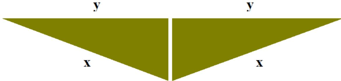
**Figure 8.4 Triangular swale cross section – divided into two right angles.**
