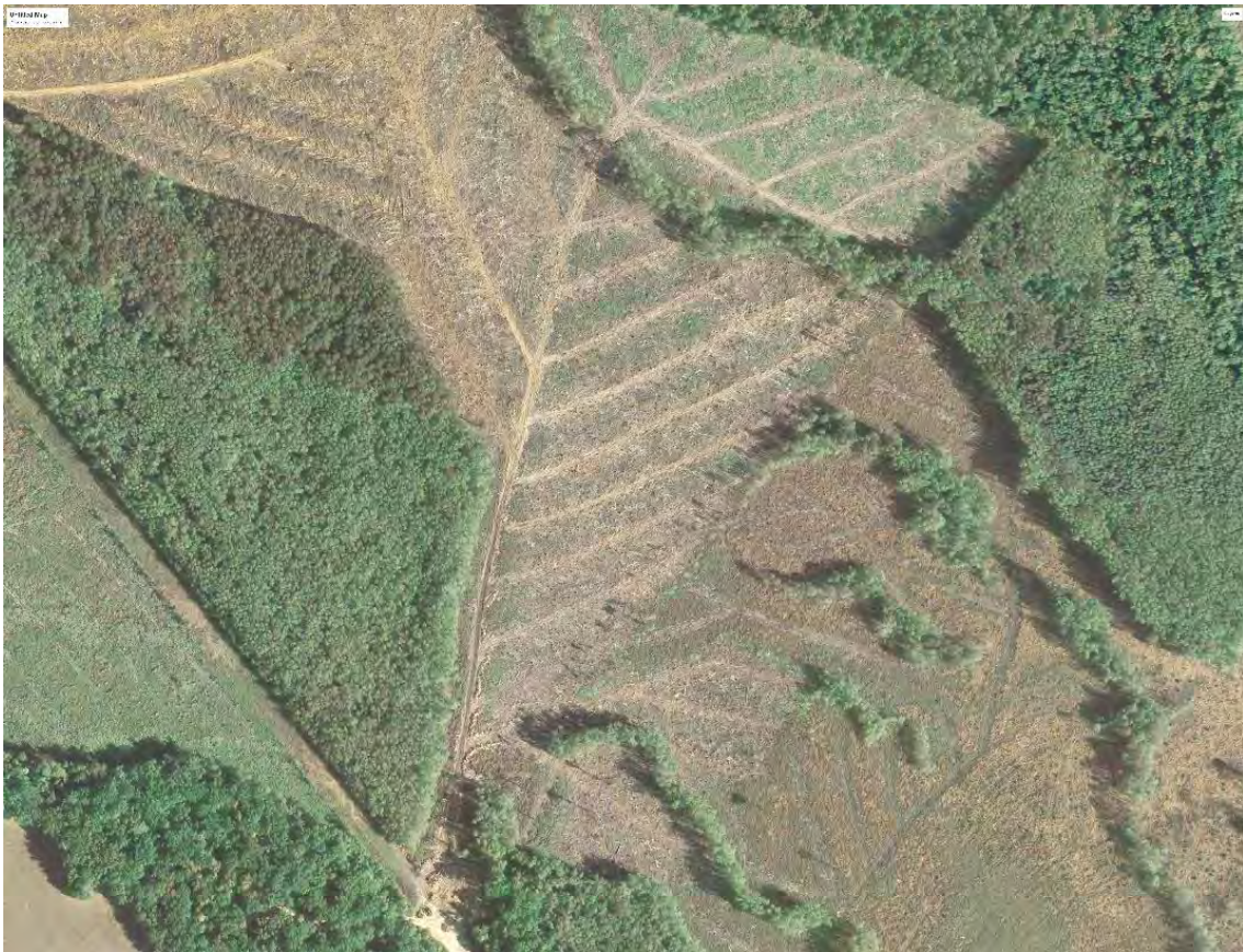
Figure 8B: Aerial view of a recently completed timber harvest using shovel logging methods Picture note: This tract was harvested using the shovel logging method. This method reduces the need to construct new logging roads, thereby minimizing potential sedimentation. (Image courtesy of Google Earth)
