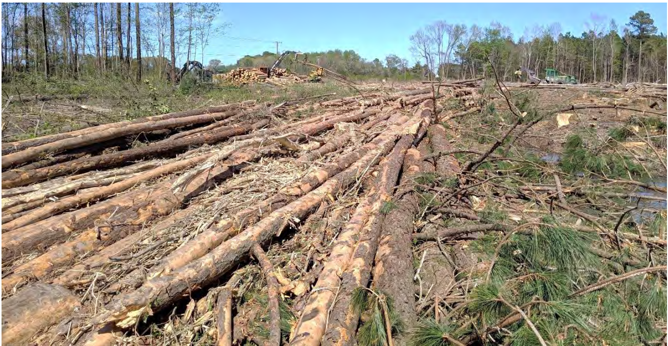
Figure 7H: A shovel trail on an active logging job in the Coastal Plain
