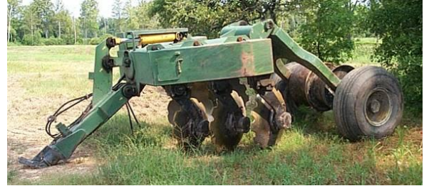
View of a typical bedding plow used in forestry.
