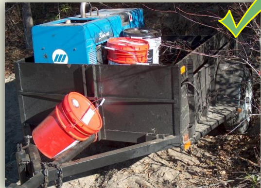
This picture illustrates well implemented BMPs for preventing waste from entering water. Equipment fluid is stored outside the SMZ and off the ground.
