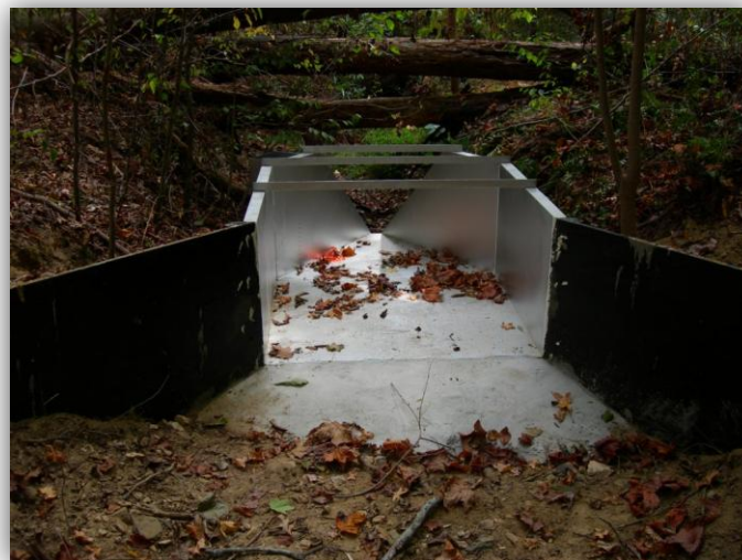
During the drought, many streams that typically flow year round were without water. This H-flume is located on a perennial stream in the Piedmont of North Carolina and was installed to monitor streamflow and water quality as part of the NC BMP Effectiveness Monitoring Watershed Study ( www.dfr.state.nc.us/water_quality/BMP_effectiveness_study.htm ).
