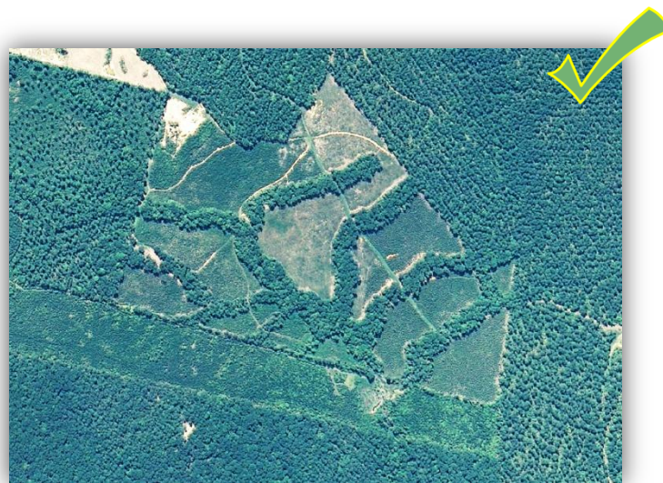
Aerial photograph illustrating properly implemented BMPs for SMZ width along streams in the Piedmont of North Carolina.
