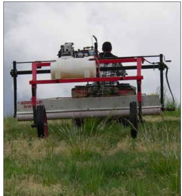
Pesticides should always be applied with care. For herbicides, equipment such as a weed wiper allows more precise application, avoiding nontarget plants and spray drift. (Photograph © Heritage Seedlings/Lynda Boyer.)
