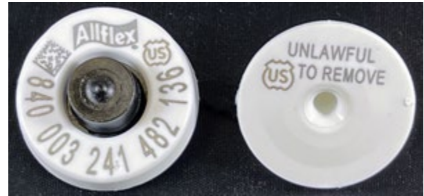
EID (electronic ID) or RFID (Radio Frequency ID) Also referred to as an “840 tag”
