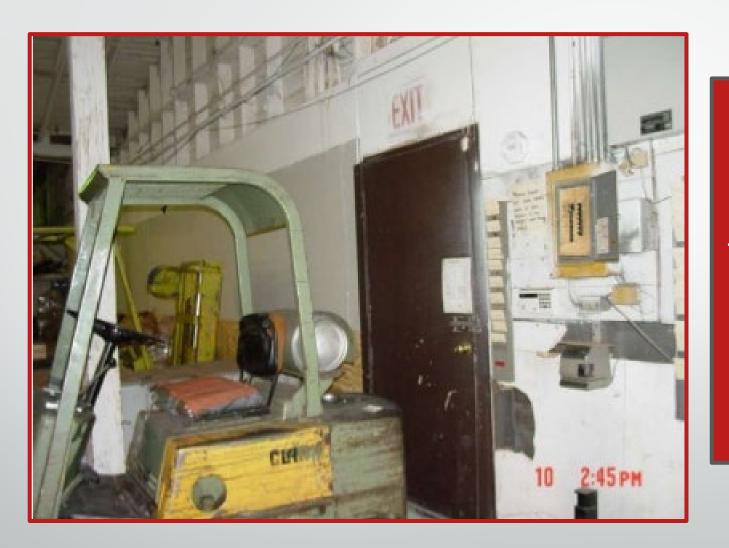
The exit door is obstructed by the forklift. This does not meet the requirements of 1910.37(a)(3)
