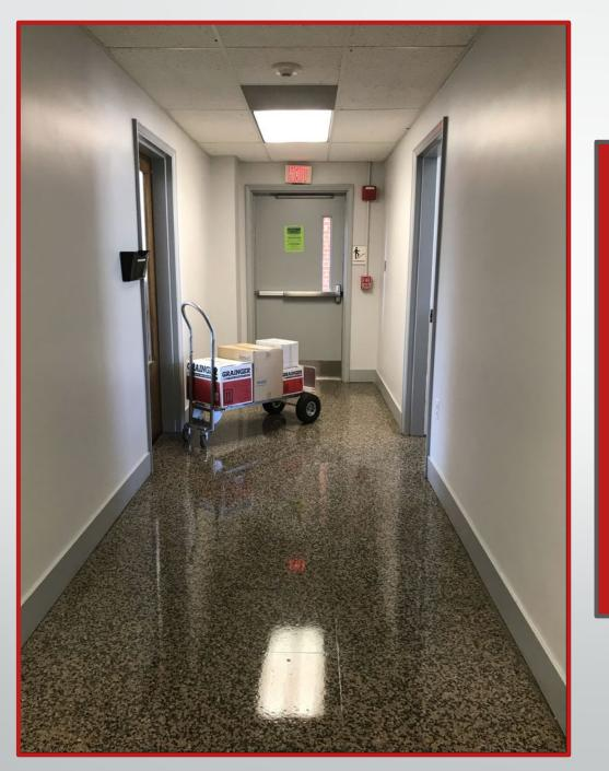
The hand cart with supplies is obstructing (blocking) the path to the exit. Therefore, the requirements of 1910.37(a)(3) are not being meet.
