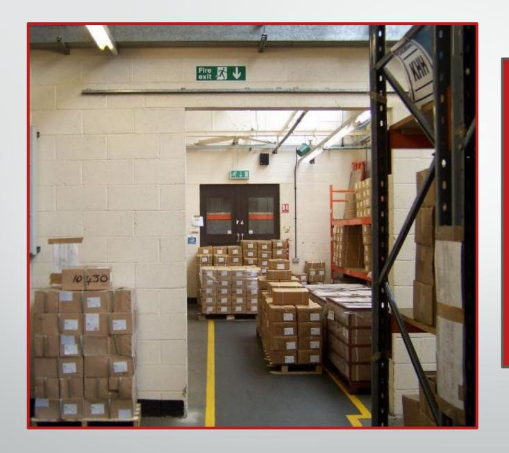
Multiple pallets of product are obstructing the exit and exit route. The yellow lines on the floor identify the exit route that must be clear.
