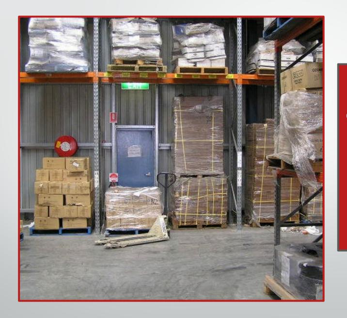
The exit door is obstructed by the pallet and pallet jack. This does not meet the requirements of 1910.37(a)(3)
