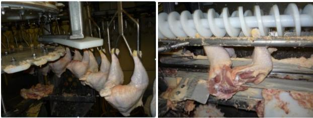
Not recommended: Sanitary operation is not being maintained. There is a significant buildup of fat and other organic material on the conveyors, blades, and associated product contact surfaces. This presents an increased risk of cross contamination.
