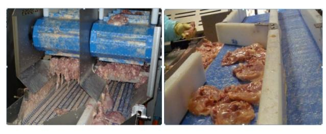
Not recommended: Sanitary operation is not being maintained. There is significant buildup of fat and other organic material on the belts. This presents an increased risk of cross contamination.
