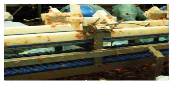
Not Recommended: Cut-up stations do not include a mechanism for cleaning knives. Knife sharpeners are available at each cut-up station and are used as needed. This set up and practice increases cross-contamination.
