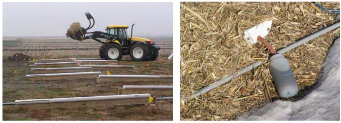
Figure 1. Gravity flow leachate collection troughs (left) and polyethylene leachate bottles (right) used to capture leachate samples during trials 5 and 6.
