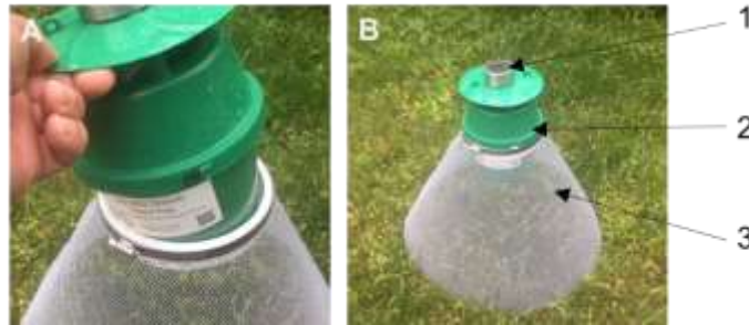
Figure 2. Details of the sweetpotato weevil trap to use in the MAT. The base of the trap is a funnel made with galvanized mesh (3). This allows weevils to walk to the bucket trap fitted within a PVC ring that holds the funnel (2). The bucket trap includes a solar cell (1) that charges an LED diode that produces a green light shown to attract more weevils. The diode is activated late in the evening when weevils are active and deactivated when there is sunlight.
