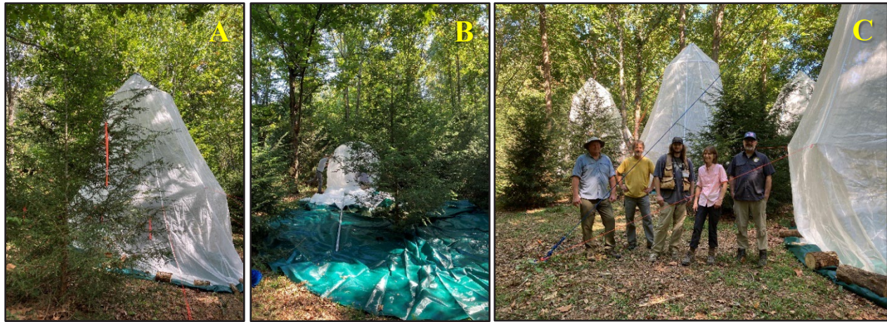
Figure 2.4. Whole-tree cage study site: A) caged tree next to uncaged control tree, B) hemlock with cage floor installed around tree base, C) NCD&CS Plant Industry staff after completion of cage installation at study site (left to right-Bill Foote, Charles Dial, Chandler Purser, Martha Flanagan, Greg Wiggins), September 2022.
