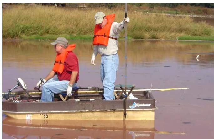
Figure 5. Sludge Judge use in an animal lagoon (Source: Field Demonstration of the Performance of Wastewater Treatment Solution [WTS®] to Reduce Phosphorus and other Substances from Dairy Lagoon Effluent. 2009. Texas Water Resources Institute)
