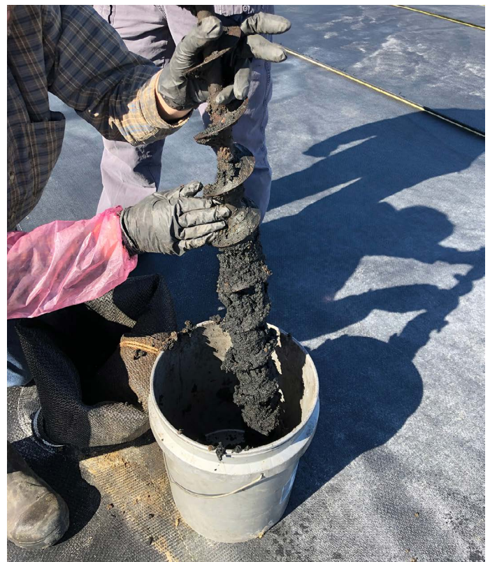
Figure 12. Sludge sampling from sludge bag port using an auger.
