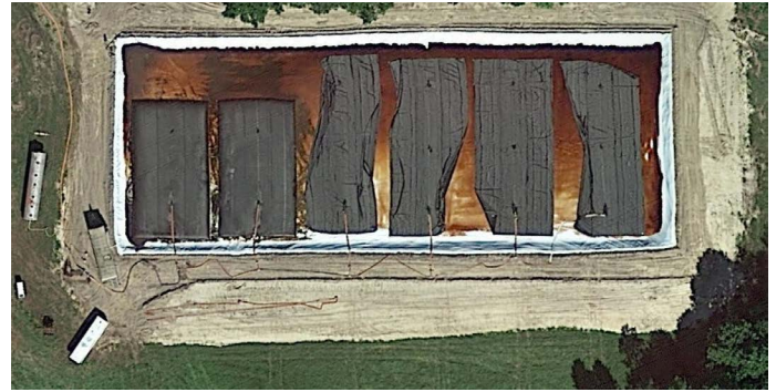
Figure 4. Sludge has been dredged and pumped into permeable bags that leach out the liquid into a lined basin. That liquid is then pumped back to the lagoon. (Source: Google Earth. 2018 satellite image from Duplin County, North Carolina)
