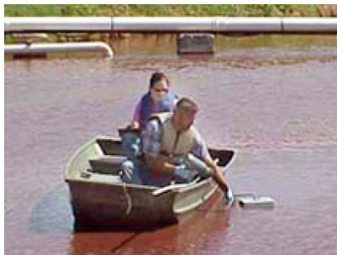
A sludge survey begins in a swine lagoon with two people in a flat-bottomed boat. The man holds a Sludge Gun, a Sludge Judge rests beside him, and a sonar device floats beside the boat.
