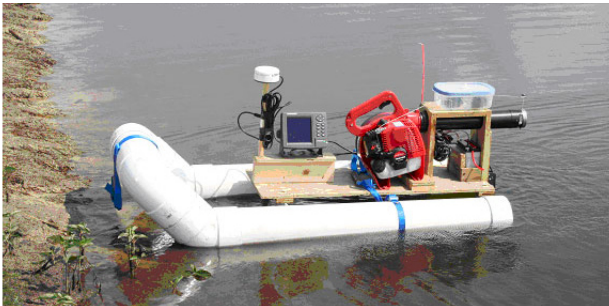
Figure 3. Remotely controlled sludge survey boat designed and built by Dan Bailey (Extension Agricultural Agent, Sampson County) utilizing a fish finder, GPS, and a gas-powered leaf blower for propulsion.
