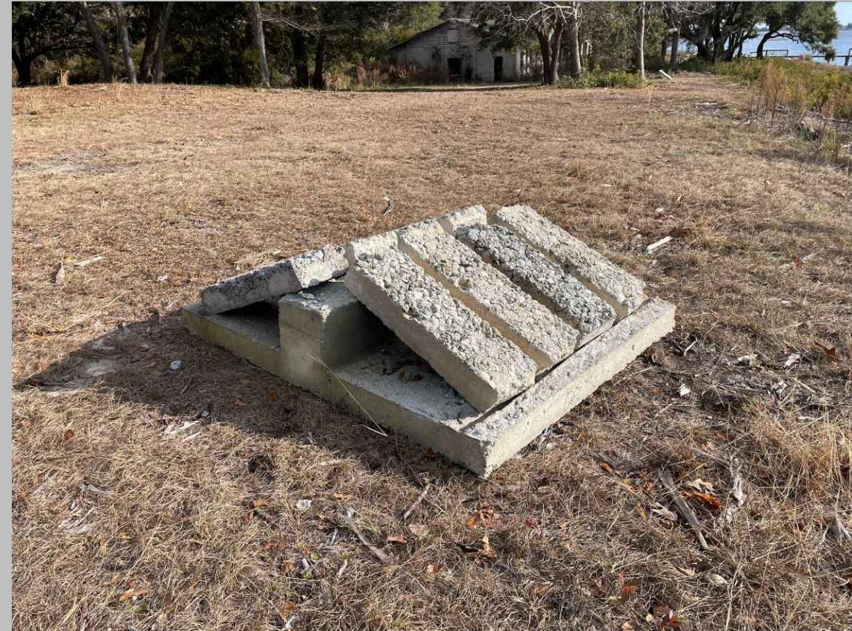
This photo shows the foundation and breakwater slabs used on the marsh sill/living shoreline project
